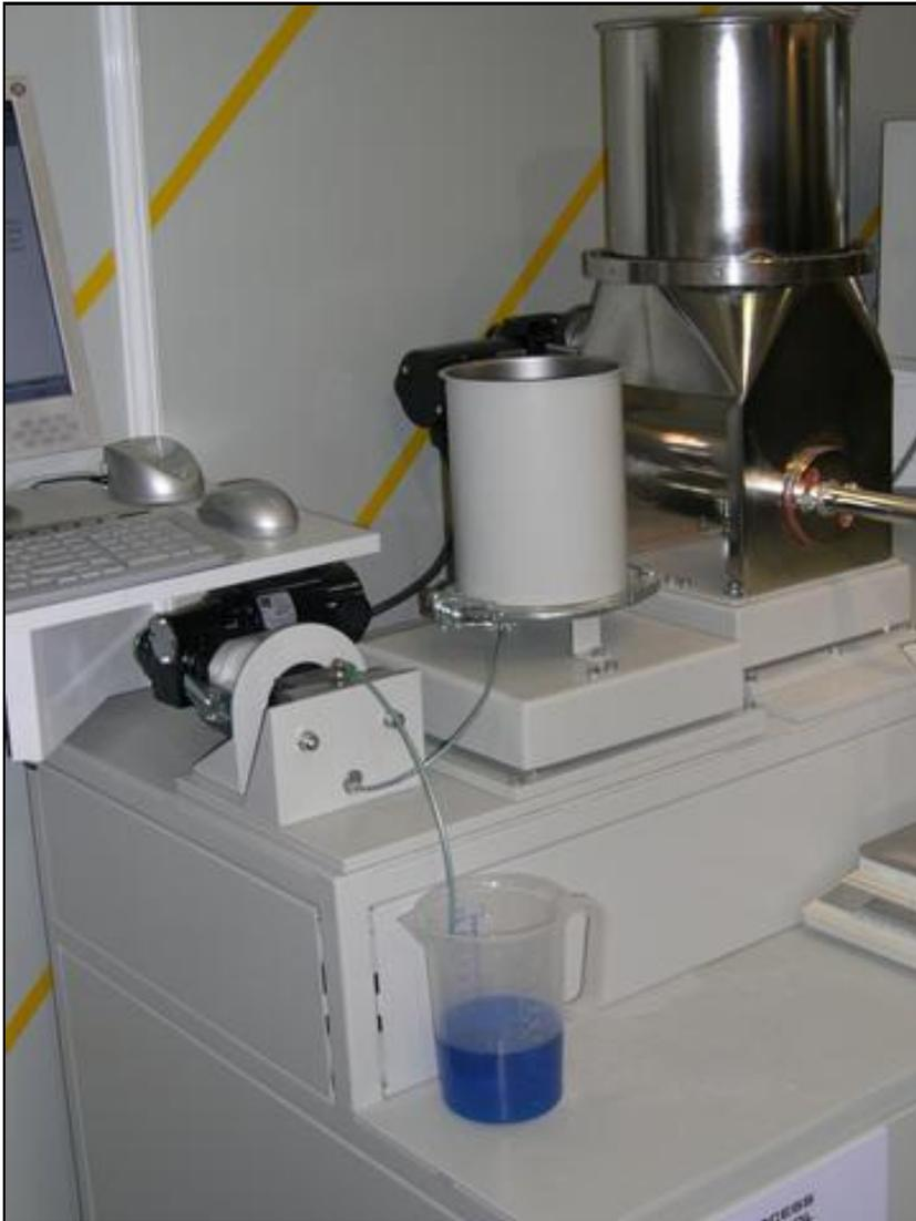
**Gravimetric Liquid Feeder LF-Series. Shown above:
