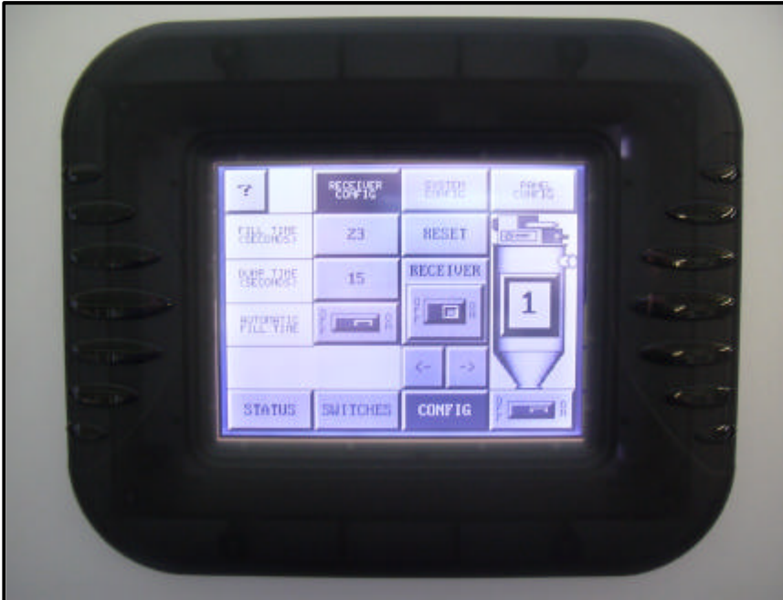
The „Director®“-Series: automatic control of vacuum conveying systems
