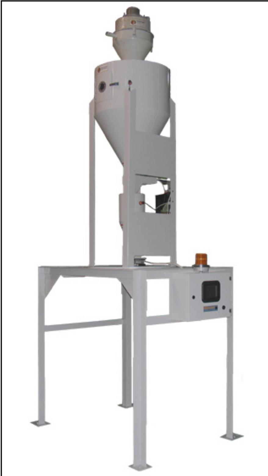
With an Inventory Control Unit it is possible to measure the unknown throughput of a process. Two operation modes are available:
