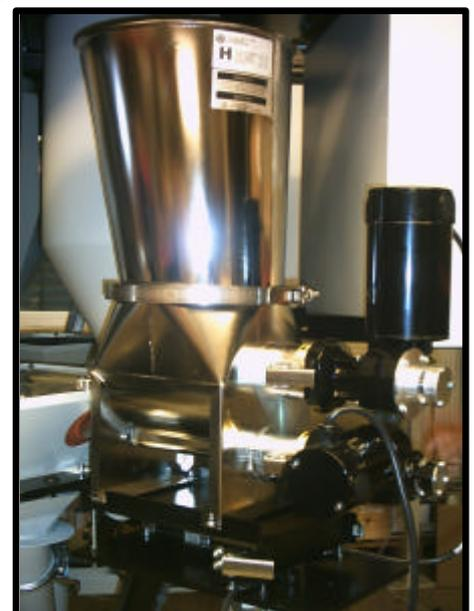
**PF Series Powder Feeder as an element of a gravimetric blender**
