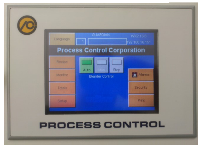
Control Panel Mini-Op B&R Touchscreen
